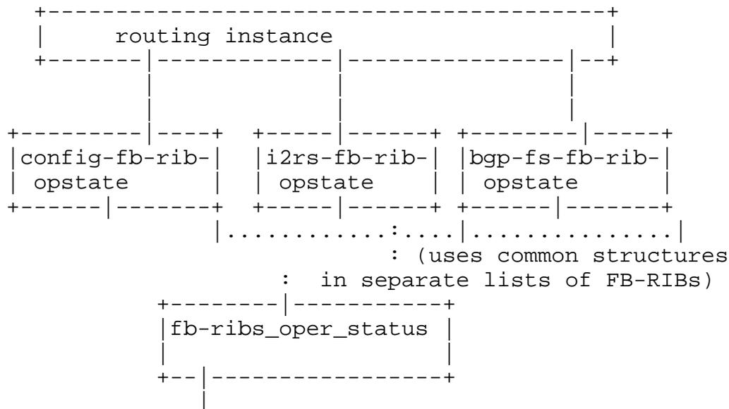
Figure 4: Routing instance with three types of Filter-FIB lists
