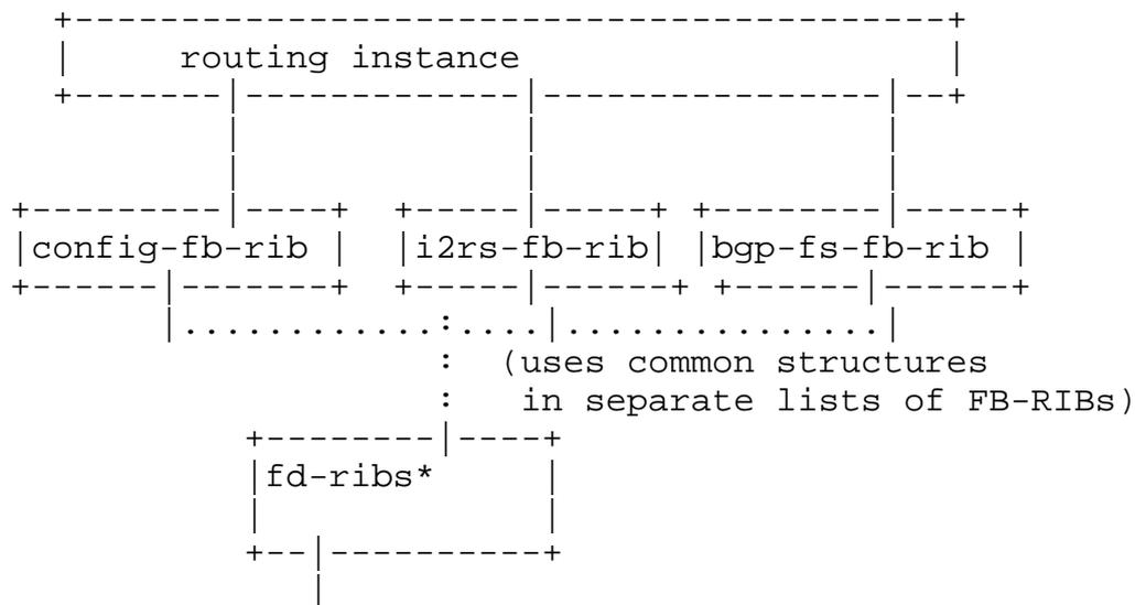
Figure 3: Routing instance with three types of Filter-FIB lists
