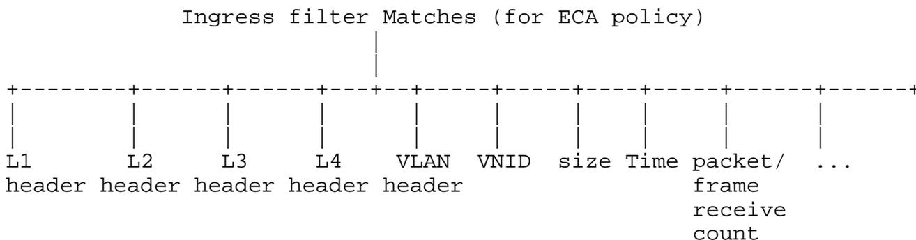
Figure 1: Possible matching conditions for basic network filters
